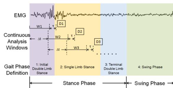
Fig. 2. Continuous windowing scheme for real time pattern recognition and definition of gait phases. For each analysis window (W1, W2, and W3), a classification decision (D1, D2 and D3) is made  $\Delta t$  seconds later.  $\tau$  is the processing time required of the classifier, where  $\tau$  is no larger than  $\Delta t$ .
