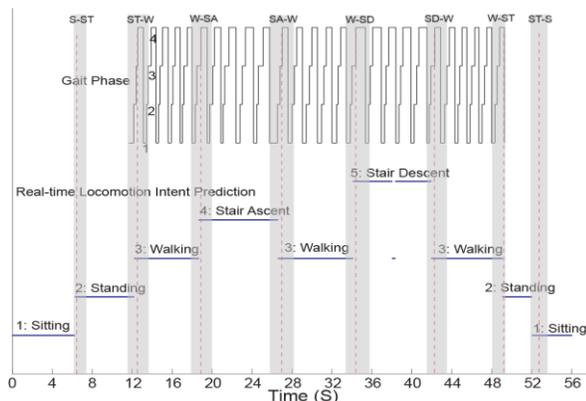
Fig.4. Real-time recognition results in one representative testing trial. The white area denotes the static states period; the gray area represents the transitional period. The red dash line indicates the critical timing for each transition.
