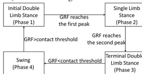
Fig. 3. The real-time gait phase detection criteria.
