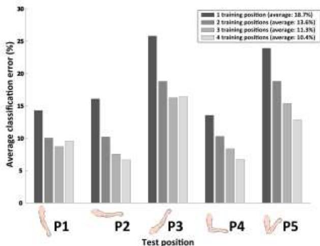
Fig. 2: Comparison of classification errors when testing in one limb position and training in all possible subsets of the remaining positions (the “Leave-one-out” strategy, as described in the *Methods* section, part E). Note that the training sets have been scaled so that they have identical size every time; independently of the number of training positions, by using subsets of the ten trials.
