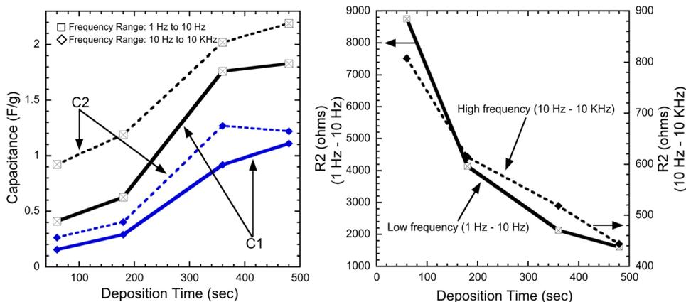
FIG. 3. (Color online) Plots as a function of g-CNT deposition time based on EIS analysis for (a) Capacitance, double-layer ( $C_1$ ) and pseudo-capacitance ( $C_2$ ) and (b) charge transfer resistance ( $R_2$ ).
