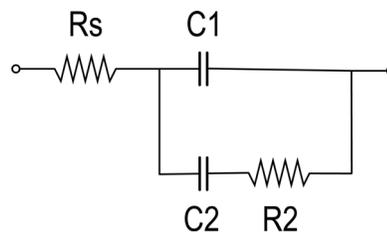
FIG. 2. Equivalent circuit model used for EIS analysis of electrode-electrolyte interface.  $R_s$  represents the solution resistance,  $C_1$  the double-layer capacitance due to linear edge defects,  $C_2$  the Faradaic pseudo-capacitance, and  $R_2$  the charge transfer resistance.
