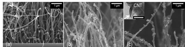
FIG. 1. SEM micrographs of the graphenated CNTs as a function of deposition time. The foliate density increases as a function of deposition time (a) 180 s, (b) 360 s, and (c) 480 s (Inset: TEM of graphene foliate showing hollow CNT core. Foliate indicated by the arrow. Scale bar is 100 nm.)
