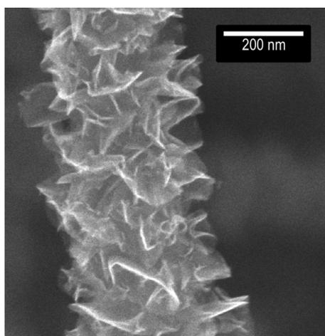
FIG. 4. SEM of an ultra high foliate-density graphenated CNT.
