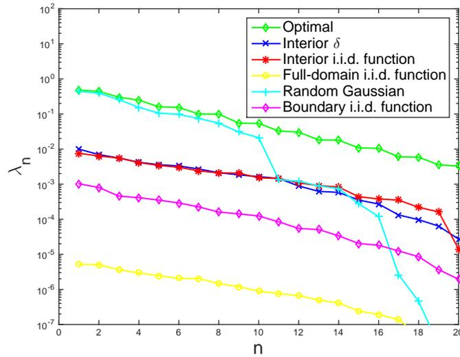
FIGURE 5.2. Eigenvalues obtained from the five different random sampling strategies, using 20 samples each, and the leading 20 eigenvalues from the reference solution. Eigenvalues are computed from (3.2) for the random sampling strategies and (2.17) for the reference solution. All methods show almost exponential decay of the eigenvalues, with the Random Gaussian strategy doing best at matching the reference eigenvalues.
