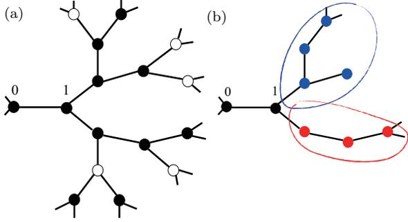
FIG. 1. (a) Sketch of a fragment of a Bethe lattice with  $z = 3$  with occupied (full circles) and unoccupied (empty circles) sites. A tracer on site 0 connects to one of the branches through site 1. (b) A sketch of a cluster branch of size  $s = 8$ . This branch can be further decomposed into two sub-branches of sizes  $s_1 = 4$  (blue) and  $s_2 = 3$  (red) connected by site 1.
