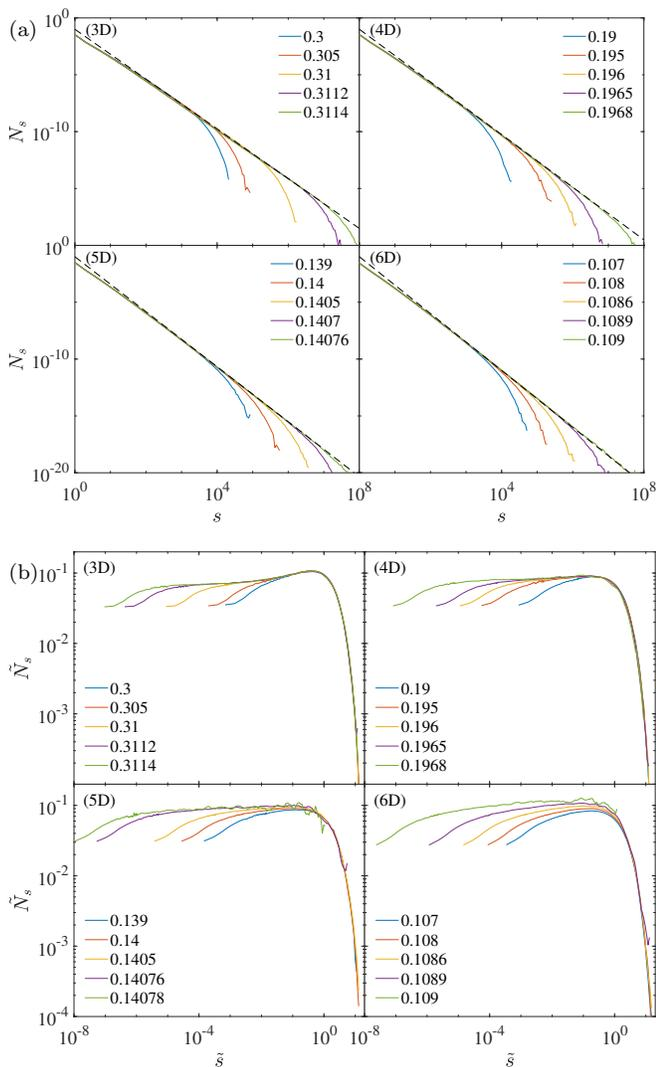
FIG. 2. (a) Cluster size distributions,  $N_s(s, p)$ , for different  $p < p_c$  in  $d = 3, 4, 5, 6$  (as given in panel labels). The Fisher power-law scaling (dashed line) describes well the large-cluster regime. (b) The rescaled cluster size distribution  $\tilde{N}_s(\tilde{s}, p)$ , shows a very good collapse for the exponential cutoff of the cluster size distribution in all dimensions, but more sizable pre-asymptotic effects for the Fisher tail can be observed as  $d$  increases.
