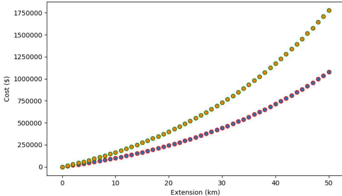
Fig. 3: Extension costs per unit distance of extension. HV-extension (Green-Yellow) costs significantly more than MV-extension (Red-Blue) over longer distances.
