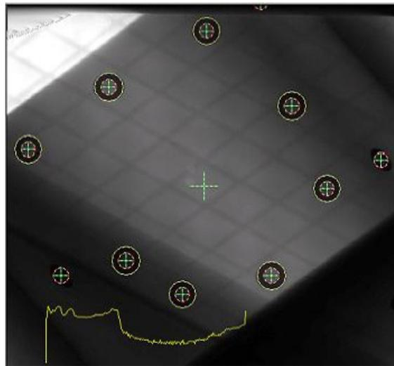
FIG. 3. An X-ray calibration phantom for daily isocenter calibration to ensure that the isocenter of the image-guided radiation therapy system is consistent with the laser system. The system reads the position of each radiopaque marker and determines the isocenter position of the X-ray system.
