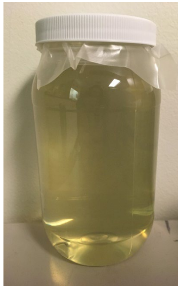
Figure 1: Fabricated NIPAM dosimeter prepared in Duke University's 3D Polymer Gel Dosimetry and Optical Bio-Imaging Lab.
