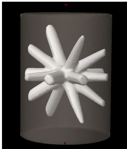
Figure 4: 3D rendering of NIPAM dosimeter and high dose volume for the isocenter verification plan, obtained from Eclipse External Beam Planning.
