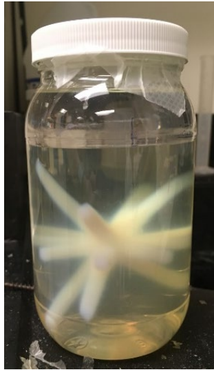
Figure 5: Irradiated dosimeter after performing the isocenter verification test using the 5 mm diameter MLCs.
