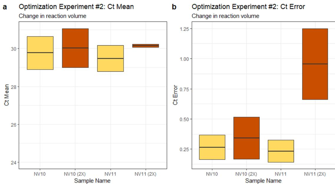
**Figure 7: Results from the second qPCR optimization experiment, doubling the total reaction volume from 12 $\mu$ L to 24 $\mu$ L. Panel A: Ct mean values per sample. Panel B: Ct error values per sample.**
