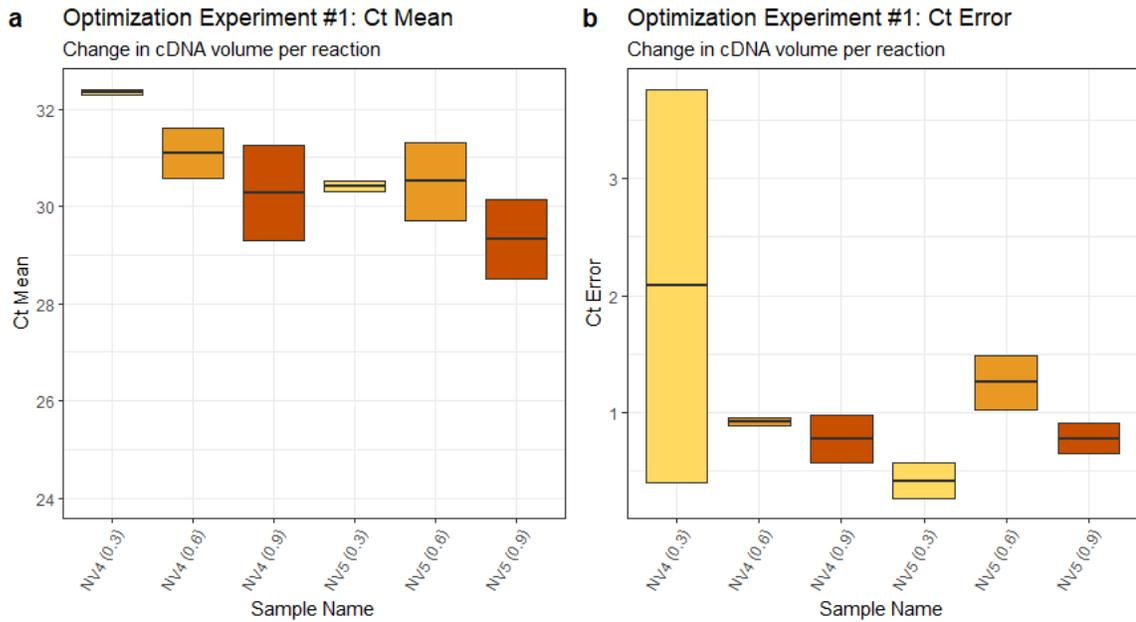
**Figure 6: Results from the first qPCR optimization experiment, changing cDNA volume from 0.3 $\mu$ L/reaction to 0.6 $\mu$ L/reaction and 0.9 $\mu$ L/reaction. qPCR was performed on two different samples at each of the three cDNA volumes specified. Light orange represents the original volume of 0.3 $\mu$ L of cDNA, orange represents 0.6 $\mu$ L cDNA, and dark orange represents 0.9 $\mu$ L cDNA. Panel A: Cycle threshold (Ct) mean values per sample. Panel B: Ct error values per sample.**
