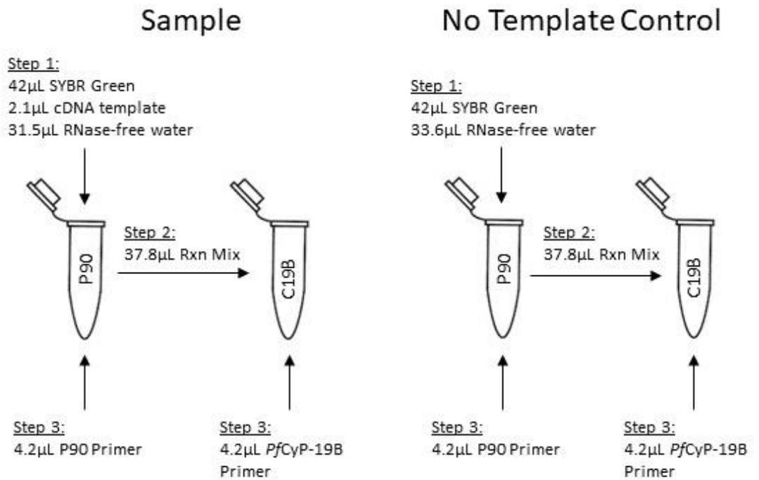
**Figure 4: Schematic of the optimized master mix workflow used for qPCR.**
