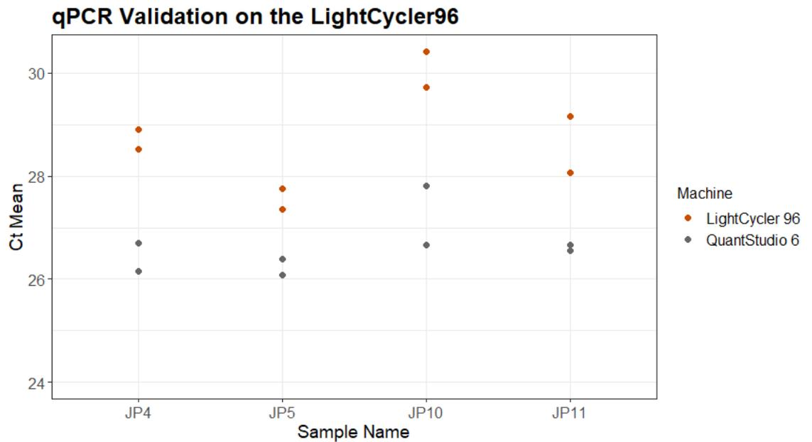
**Figure 5: qPCR assay validation on the LightCycler®96. Four samples underwent qPCR on two real-time PCR machines. First, the QuantStudio 6 and later the LightCycler®96. Cycle threshold (Ct) mean values were compared between the two machines.**
