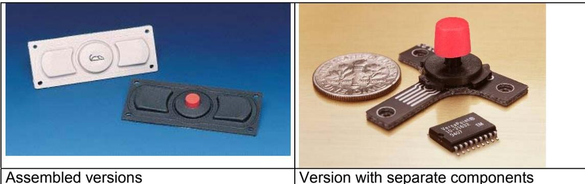
In addition to the version of the mini-joystick used for this project, another non-assembled version of the joystick is available, composed of the MicroJoystick, the microcontroller for sensor handling and communication with the PC and buttons, which provide maximum assembly versatility, in order to exploit the extremely limited dimensions of the single components without altering the other functional characteristics.
