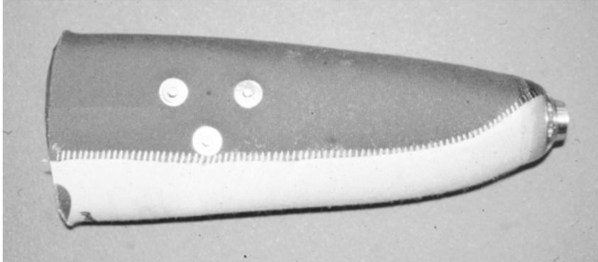
Ill 2 Stainless steel snap electrodes in a roll-on liner
