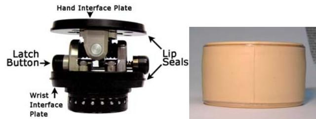
**Figure 1:** Depicts a close up view of a) MF wrist, latch button and lip seals and b) seal. The latch button engages or disengages the locking mechanism. Proximal and distal lip seals were created to allow the donning of a flexible membrane. This membrane minimizes debris, and moisture entering the MF wrist unit.
