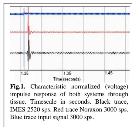
Fig.1. Characteristic normalized (voltage) impulse response of both systems through tissue. Timescale in seconds. Black trace, IMES 2520 sps. Red trace Noraxon 3000 sps. Blue trace input signal 3000 sps.
