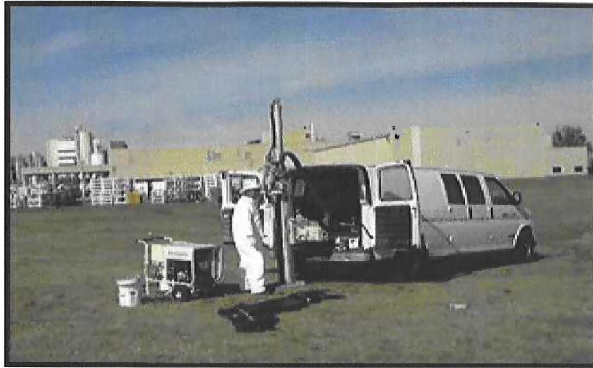
Figure 6 – Typical rig used for chemical injection programs (Source: Zebra Environmental)
