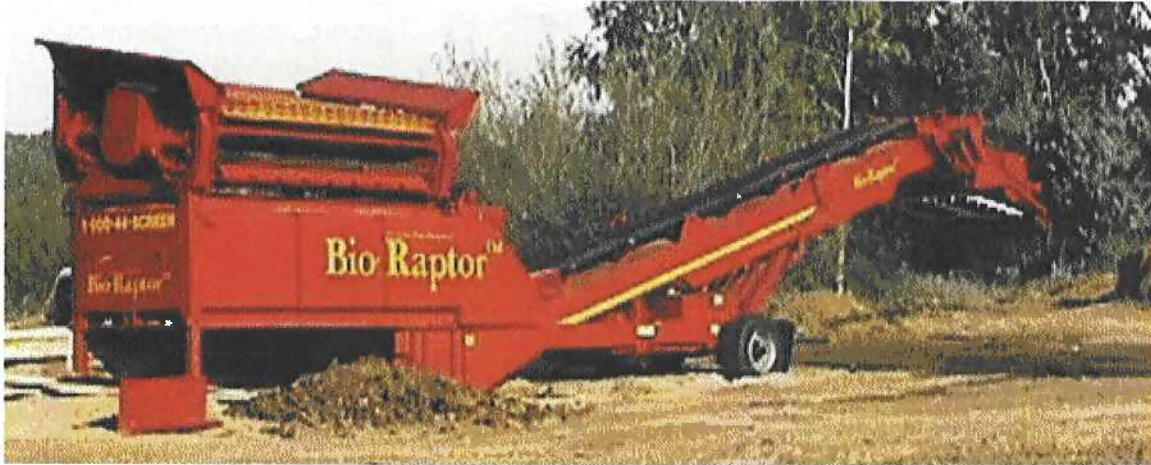
Figure 5 – Typical pug mill used for soil shredding (Source: US Microbics, Inc.)
