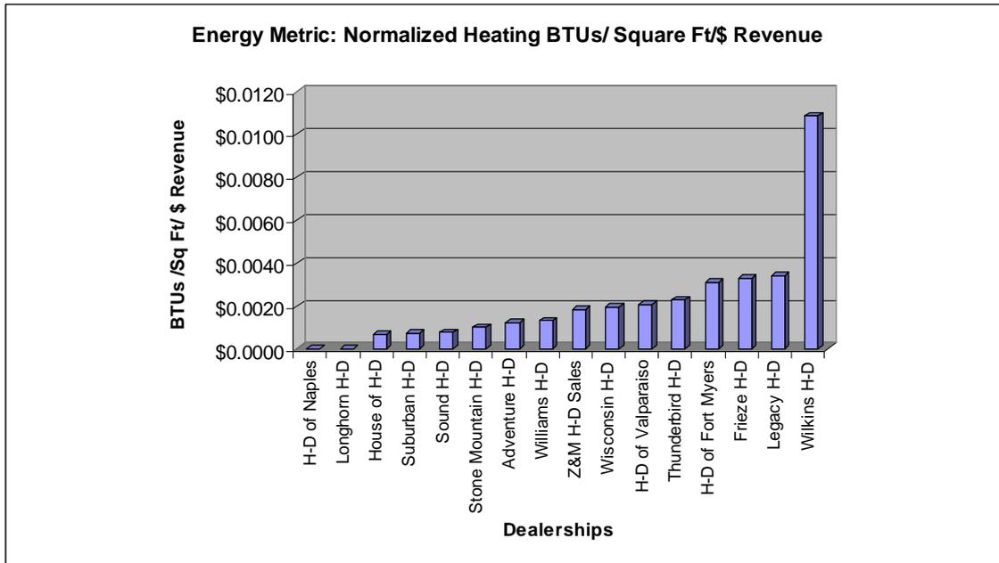
Figure 11: Heating Sub-Metric Normalized. This chart compares heating BTUs / Square foot/\$ Revenue for dealers in the survey.
