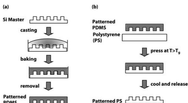
**Scheme 1** Fabrication of nanogratings. (a) PDMS nanogratings are fabricated using soft lithography. PDMS mixed with its crosslinker is casted onto the Si master. After baking the patterned PDMS is separated from the Si master. (b) PS nanogratings are fabricated using nanoimprinting. A PDMS mold is used to emboss nanogratings into the viscous PS at a temperature above the  $T_g$  of PS. After cooling the patterned PS is separated from the PDMS mold.
