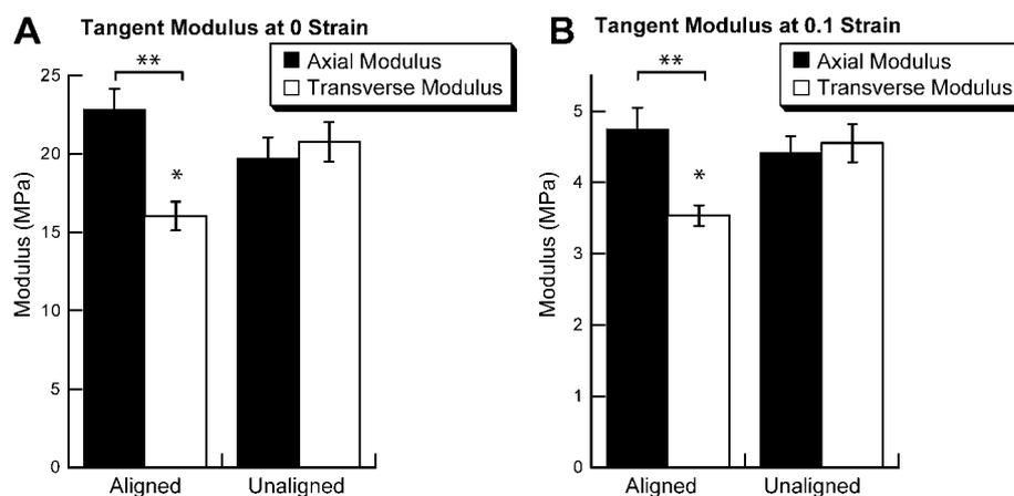
**Fig. 4** Tangent moduli at (A) 0 strain and (B) 0.1 strain for scaffolds tested in axial and transverse directions. Aligned scaffolds are stiffer in the axial direction. (\*\*  $p < 0.0005$  for 0 strain,  $p < 0.001$  for 0.1 strain.) Unaligned scaffolds, axial and transverse directions not different:  $p = 0.54$  for 0 strain,  $p = 0.70$  for 0.1 strain. \* Denotes that aligned transverse modulus is different from all other groups,  $p < 0.05$ . (Mean  $\pm$  SEM.)
