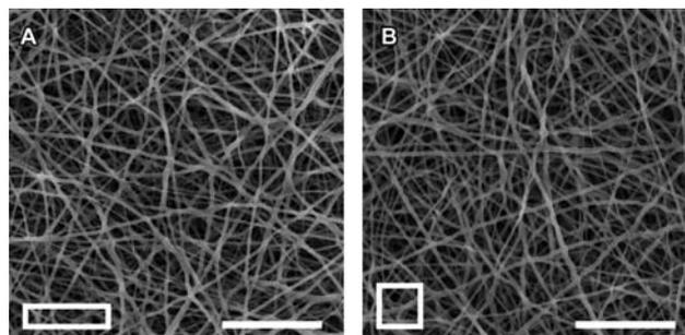
**Fig. 2** Scanning electron micrographs of scaffolds produced using (A) rectangular mask (aligned scaffold) and (B) square mask (unaligned scaffold). Expected axis is horizontal. (1000× magnification. Scale bar = 50 μm.)
