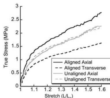
**Fig. 3** True stress v. stretch curves for representative scaffolds. Note that the axial and transverse unaligned curves are almost superimposed and the aligned scaffolds show higher stress and stiffness in the axial direction compared to the transverse direction.
