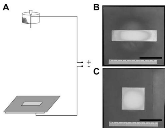
**Fig. 1** (A) Electrospinning apparatus. The copper collector electrode is covered by a rubber insulating mask with a 25 cm<sup>2</sup> aperture. (B, C) Scaffolds on collector electrode with insulating masks *in situ*. (B) Rectangular mask and scaffold. Note the small amount of fibers collected on the mask. (C) Square mask and scaffold. Scale bar = 5 cm.
