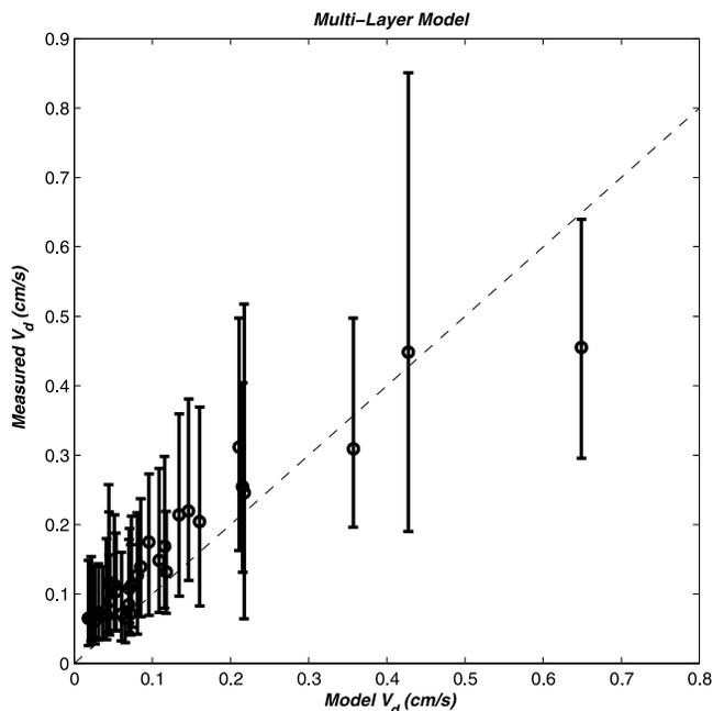
**Figure 5.** Comparison between measured and modeled  $V_d$  at  $z/h = 1.53$  for all the runs, particle diameters, and  $u_*$  conditions. The vertical bars represent 25 and 75 percentiles. The 1:1 line is also shown.
