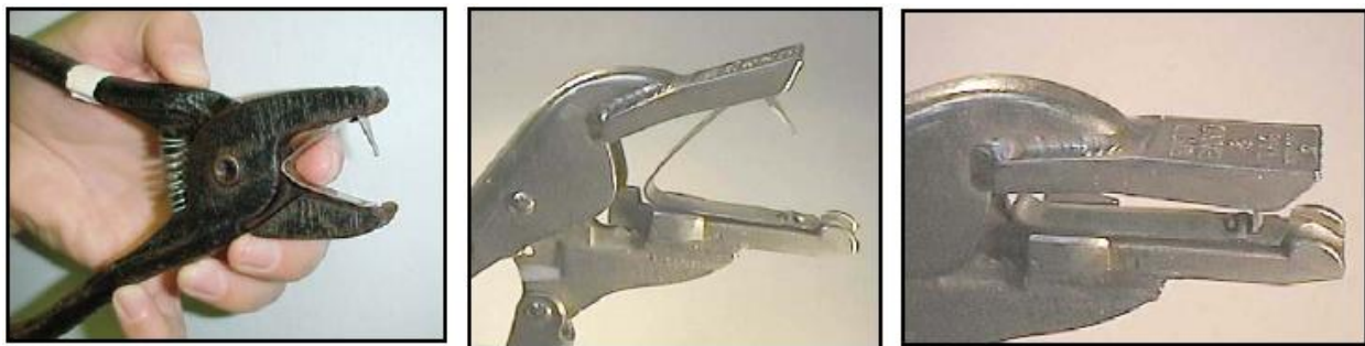
Figure 5: A Monel style 49 metal flipper tag correctly loaded (left) and cinched (right) in the application pliers. Always align the base plate of the tag flat against the pliers. Note the tine bent over and completely through the stirrup. Source: http://www.nationalband.com/nbt.pdf
