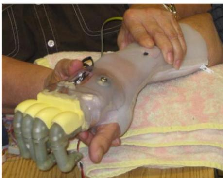
myoelectric prosthesis equipped with ProDigits developed by Touch Bionics. See figure 5
