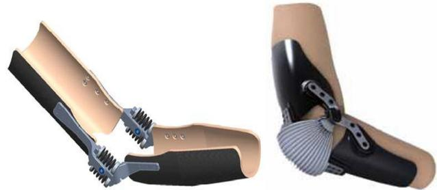
Figure 4: Design study of the OrthoJacket powered orthosis with two FFAs on each side of the elbow joint to enable both powered flexion and extension of the elbow (le.) and design with one FFA under use of pressure and vacuum (re.)
