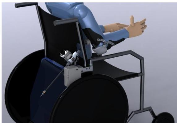
Figure 1: OrthoJacket system, mounted on a wheelchair
