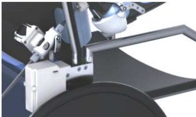
Figure 5: Shoulder module, mounted on a wheelchair
