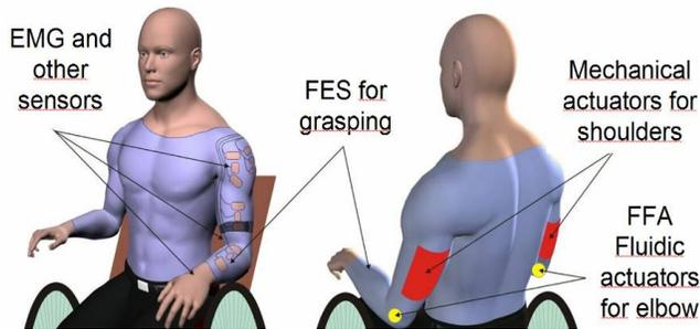
Figure 2: Relevant components of the new orthosis
