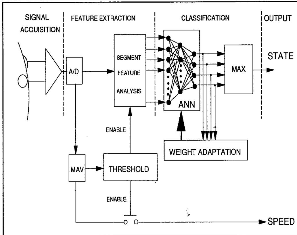
Figure 2. Control System design.
