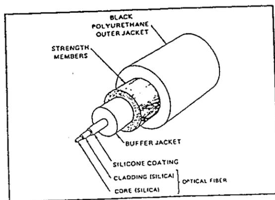
Figure 1: Typical optical fibre structure used by the communications industry.
