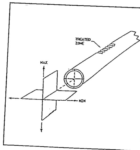
Figure 3: BEF sensor is an optical fibre with a treated strip. Planes of maximum and minimum sensitivity are indicated.
