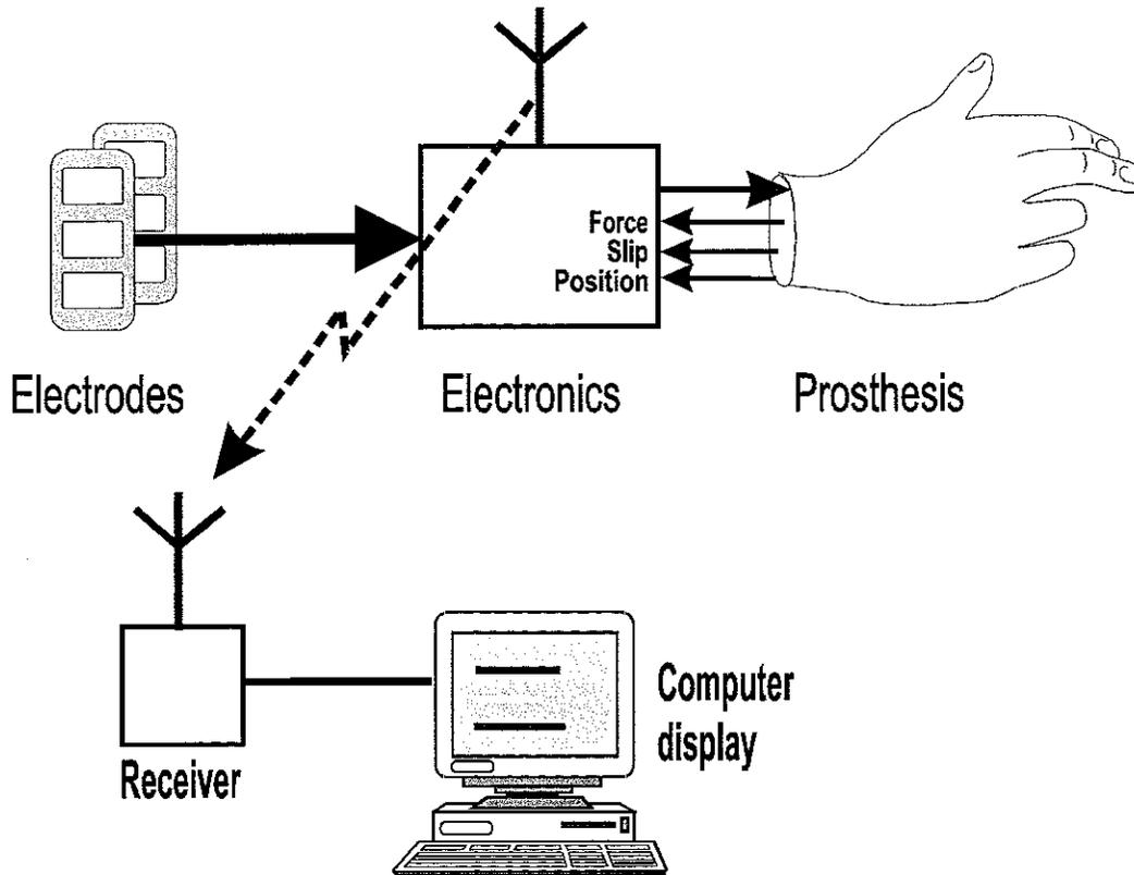
Figure 1 - Telemetry system for the LO/SH Hand
