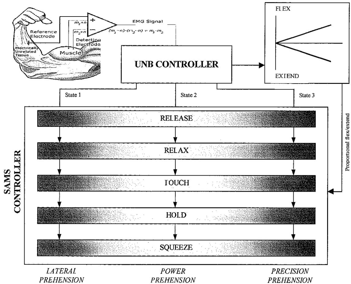
Figure 3 - Direct Prehensile Pattern and Adaptive Manipulation Control with the UNB/SAMS Controllers
