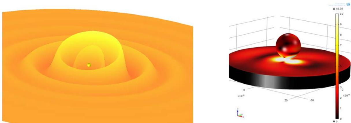
**Figure 3.** 2.5 D vector-field simulations of a gold nanoparticle held above a gold film substrate with a thin (1nm) self-assembled polymer layer [4]. Left: The surface charge wave associated with the surface plasmon polariton of the film is visualized using the Deformed Surface plotting tool in COMSOL. Right: a more conventional color surface plot showing the actual film and the particle.
