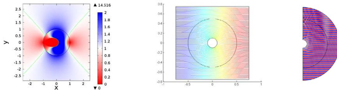
**Figure 2.** Directional cloak introduced in [1] based on the conformal mapping from Ref. [2]. Left to right: refractive index profile; ray tracing obtained with COMSOL Particle Tracing Module; 2.5D full-wave simulation based on the 3-component vector E-field formulation.
