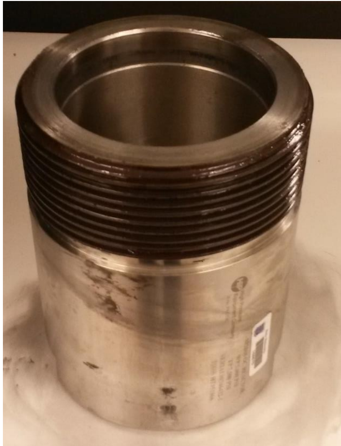
Figure 19: Pressure Vessel, Fabricated by HIP according to our design and rated by ANSI for a working pressure of 5000 psi.
