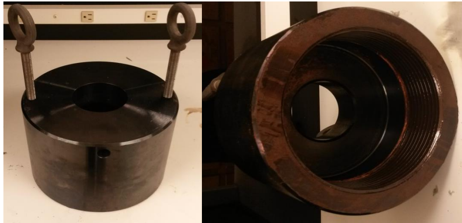
Figure 23: Cap of the pressure vessel system with bore and threading shown
