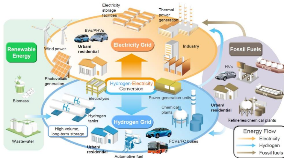
Figure 3: A flow chart depicting a hydrogen based economy with integrated renewable and conventional electricity generation (Ball and Wietschel 2009).
