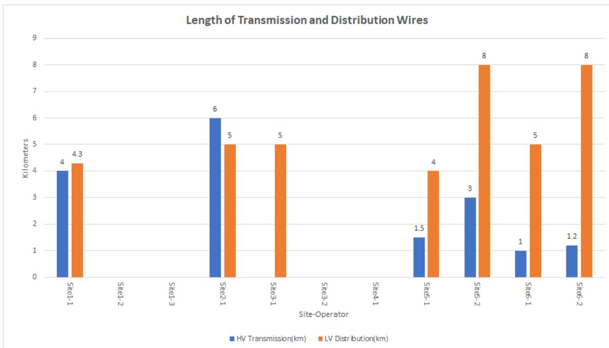
Figure 2: Length of Transmission and Distribution Wires. Data sourced from operator interviews. Disagreeing numbers for same site or the lack of numbers is to be noted.
