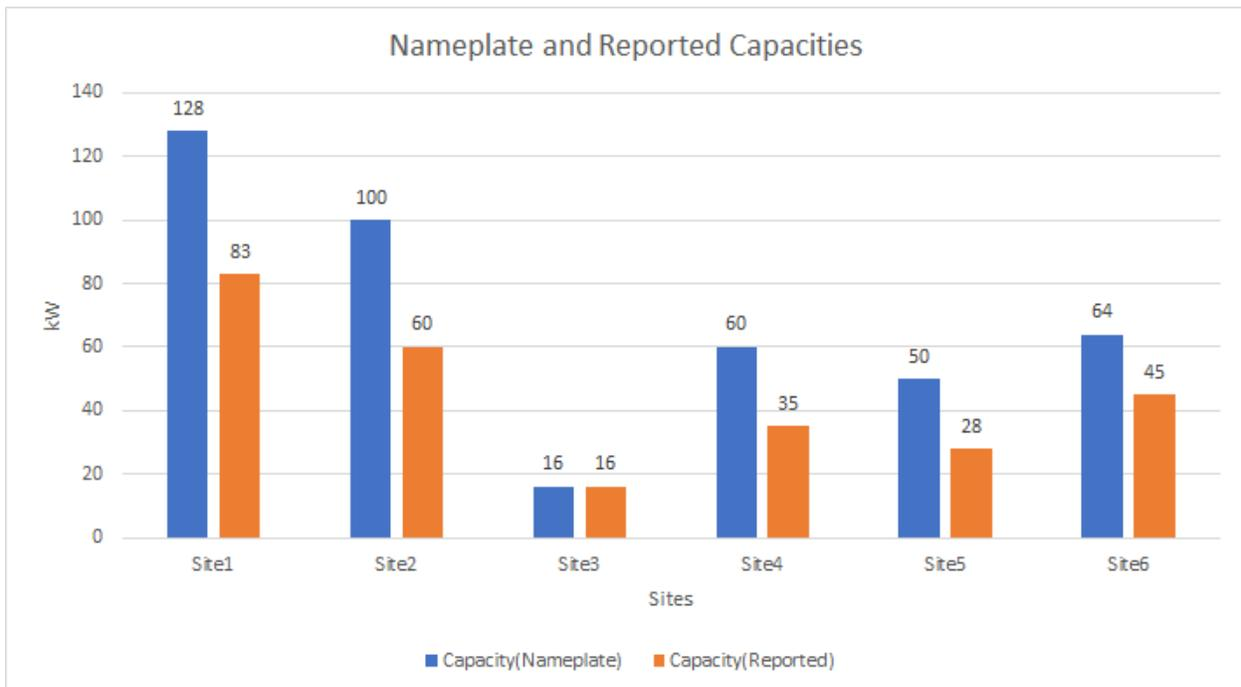
Figure 7: Nameplate Capacity and Capacity Reported by Operators. Data sourced from Operator Interviews.
