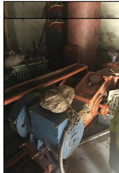
Images 3 and 4: Dangerous Solution to Equipment Malfunction. Images Taken while onsite.
