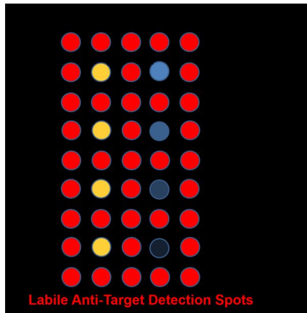
Figure 38: Test array format. Each stable capture spot is surrounded by labile detection spots in order to reduce diffusion distance of detection antibodies.
