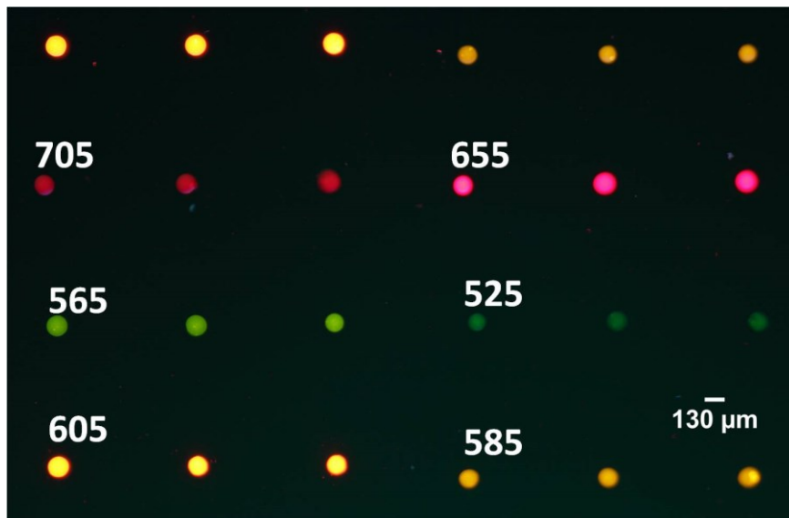
Figure 35: Demonstration of multicolor imaging of a test array printed using quantum dots of various emission wavelengths (labeled with the manufacturer quoted emission wavelength for each type of quantum dot used in array).
