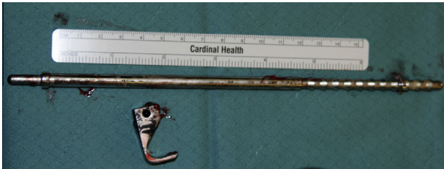
Fig. 3. Harrington rod and distal hook after removal. (For interpretation of the references to colours in this figure legend, the reader is referred to the web version of this paper.)
