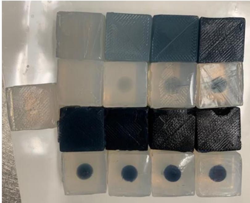
Figure 3: GNS phantoms used for laser delivery experiments. In order from top to bottom: 1 st and 3 rd rows are homogeneous phantoms, 2 nd and 4 th rows are heterogeneous phantoms (Photo Credit: Aidan Canning)
