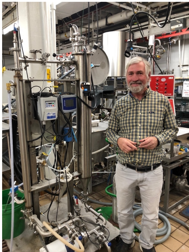
Figure 7: Sheppard in front of the yeast propagator that he built at NC State's brewery.
