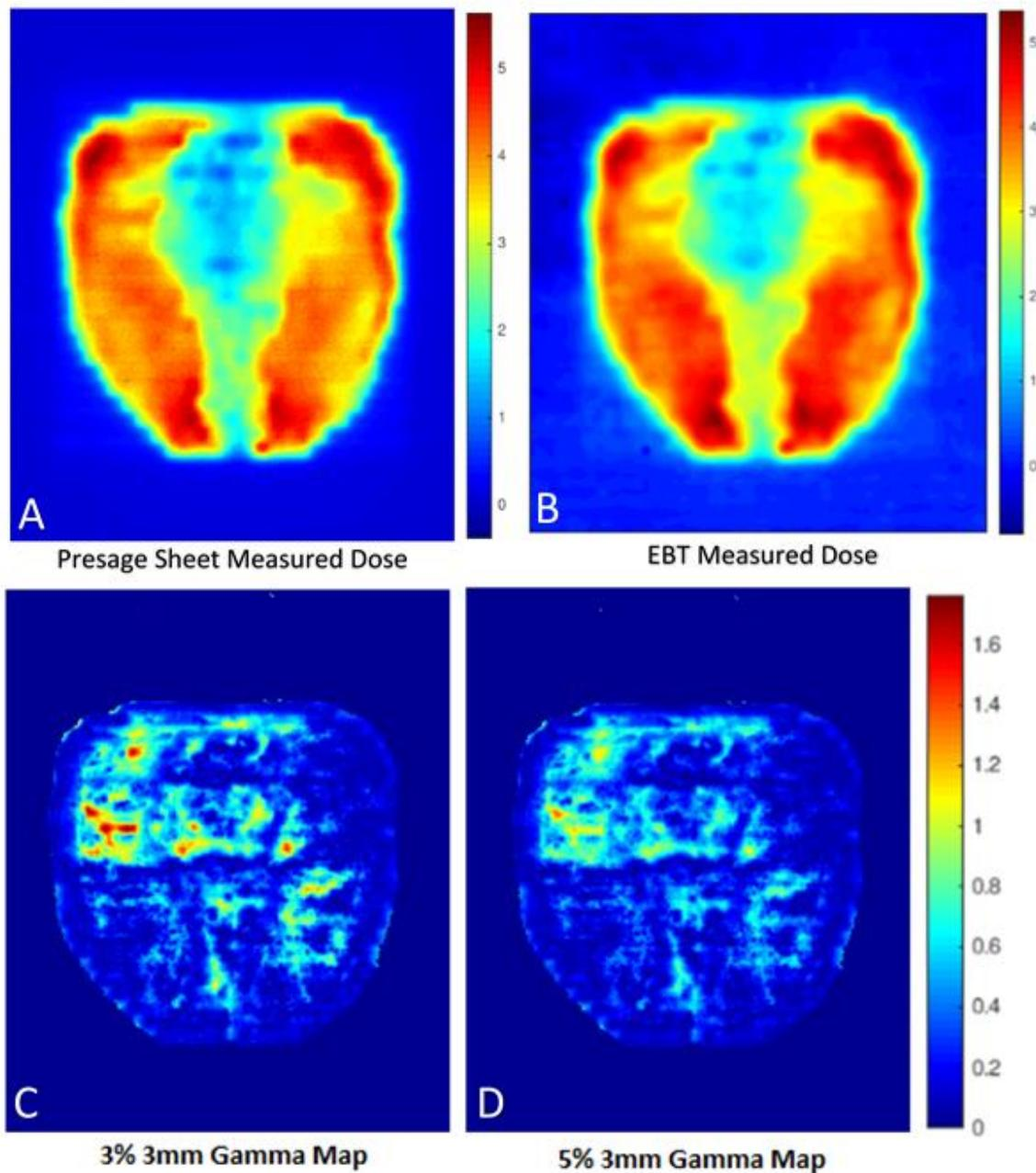
Figure 10: IMRT QA Prostate plan delivered to both the reusable Presage sheet (A) and an EBT film (B). The gamma map comparison between the two measurements at 3% 3mm yielded a 97% pass rate in the IMRT field region (C) and the comparison at 5% 3mm yielded a 99% pass rate (D).
