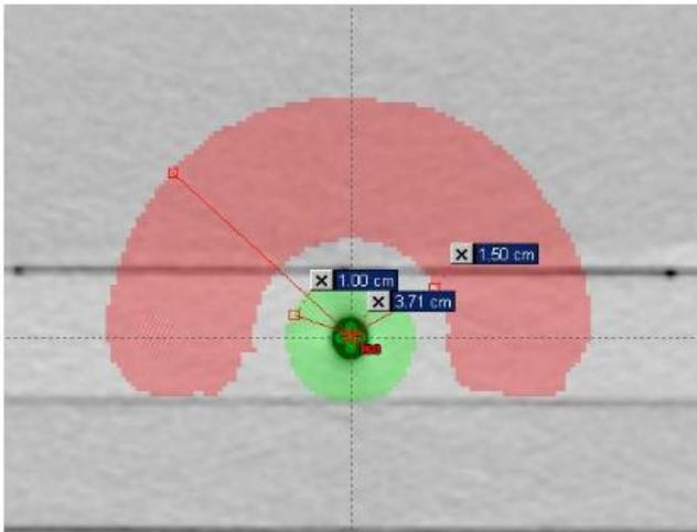
Figure 2: Prompt and illustration of TG-119's C-Shape test for IMRT commissioning using radiochromic film and a solid water phantom to test the capabilities of the IMRT delivery system.
