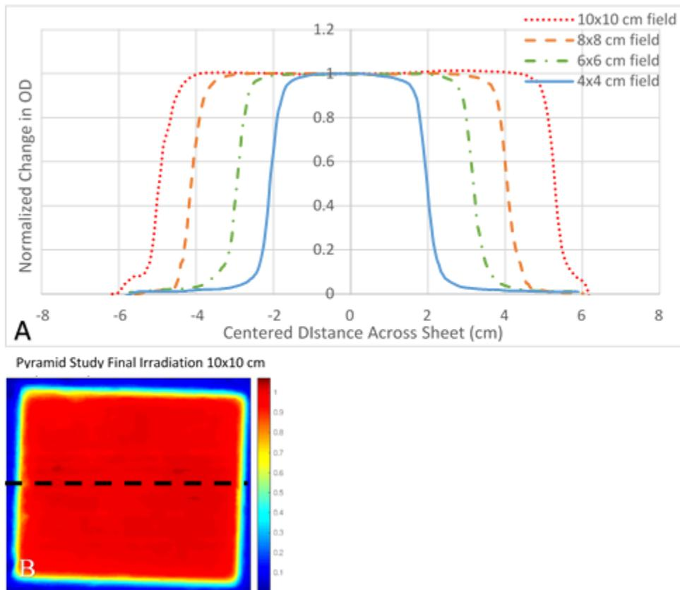
**Figure 7: Pyramid reusability test. The plot presents line profiles through the center of the pyramid irradiation field shown in figure 6. Each irradiation delivered 4.5 Gy to the sheet. (B) is a color-map of the final pyramid irradiation dose distribution, line profile indicated in black dashed line.**
