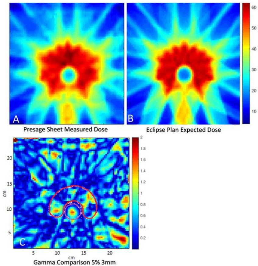
Figure 13: TG-119 C Shaped test for IMRT commissioning. (A) is the delivered color-map dose pattern in the Presage sheet. (B) is the Eclipse plan color-map. (C) is
