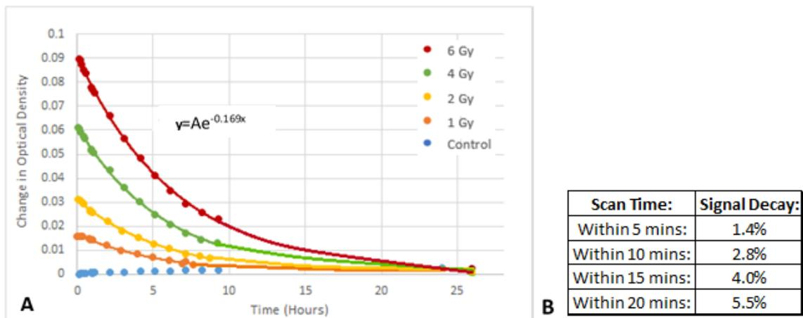
**Figure 5: Temporal decay of single irradiated Presage signal in a 26 hour period. Five different sheets were irradiated to four doses. Decay is well modeled by exponential decay,  $R^2 = 0.9986$ . The formula for the decay is displayed in the image with A representing the amplitude of decay, which is dependent on the irradiation**
