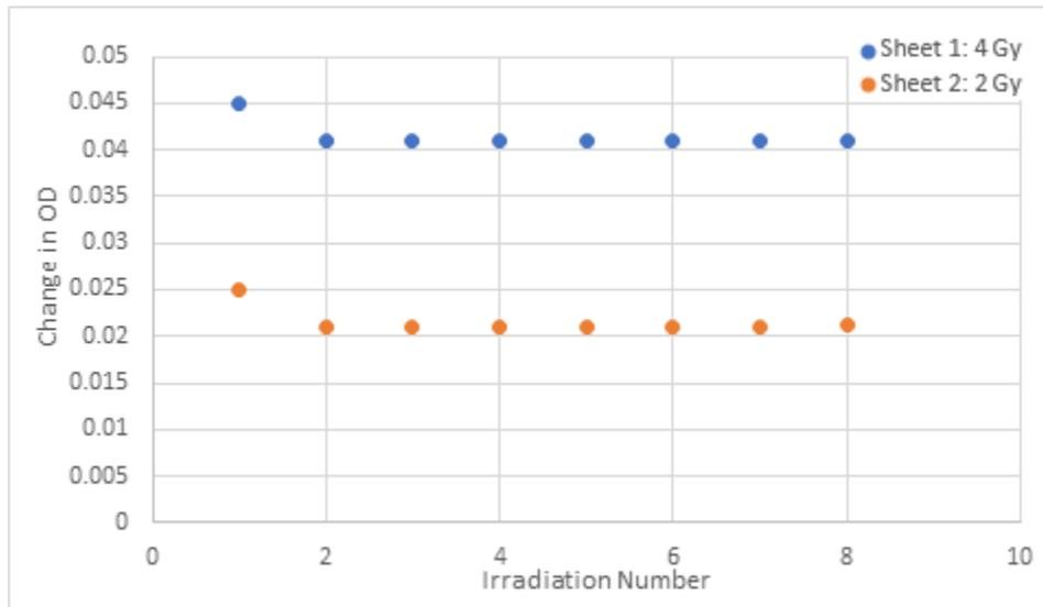
**Figure 8: Consistency of signal upon repeated irradiation. The same reusable Presage sheets were irradiated with a 30x30cm field to 4 Gy on 8 different days (blue) and a different sheet to 2 Gy for the same duration (orange). Signal was read at 10 minutes post-irradiation.**
