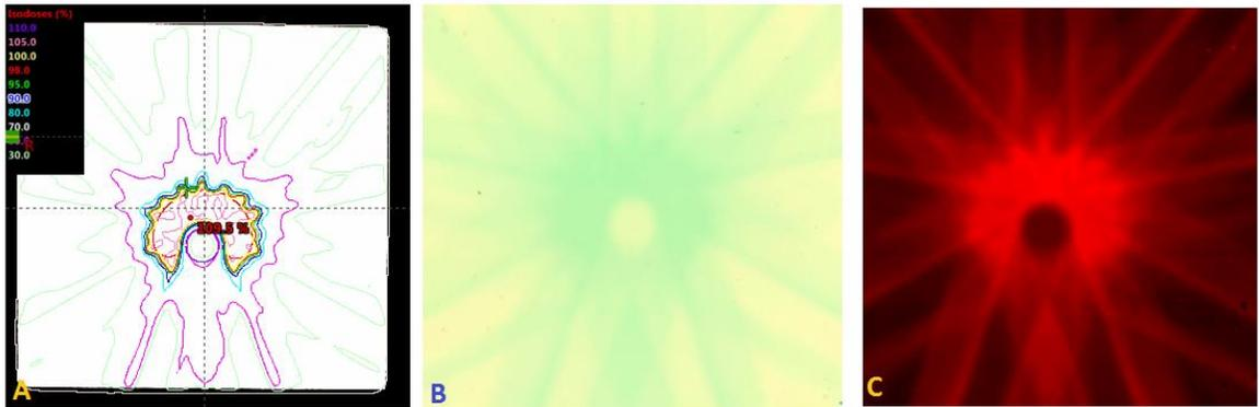
Figure 12: (A) pictures the TG-119 C-Shape IMRT treatment plan. (B) is the reusable Presage sheet readout scan. (C) is the red channel of the RGB readout scan, which is used for analysis.
