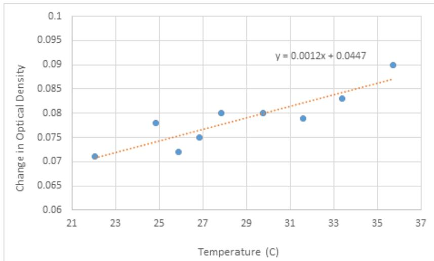
**Figure 9: Reusable Presage optical density dependence on temperature at the time of irradiation. Temperatures from 22°C (cool room temperature) to 36°C (two degrees above typical skin temperature) were tested. The orange line represents the trend line for the change in OD measurements as sheet temperature varied.**
