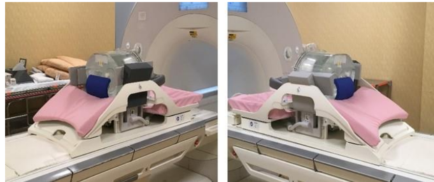
Figure 21: Phantom setup for the prone-only MR scan using the Sentinelle breast coil and Siemens Skyra scanner.
