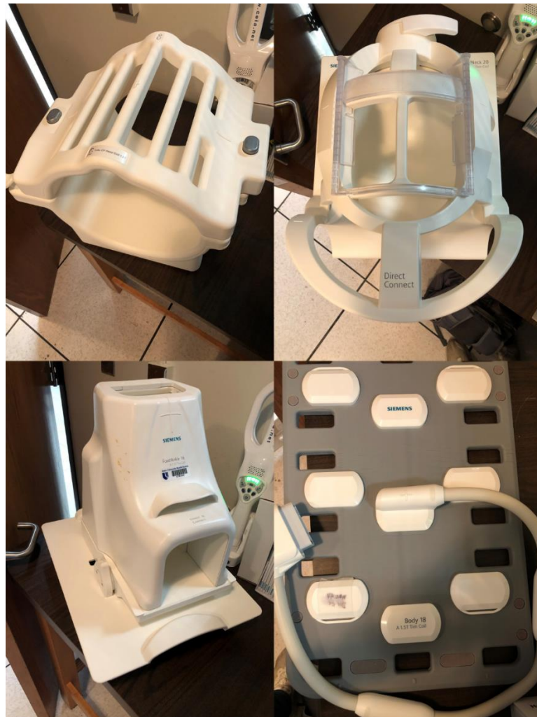
Figure 1: Anatomy specific coils in clinical use. Clockwise from top left: transmit/receive head coil, receive only head coil, foot/ankle coil, and flexible body matrix coil
