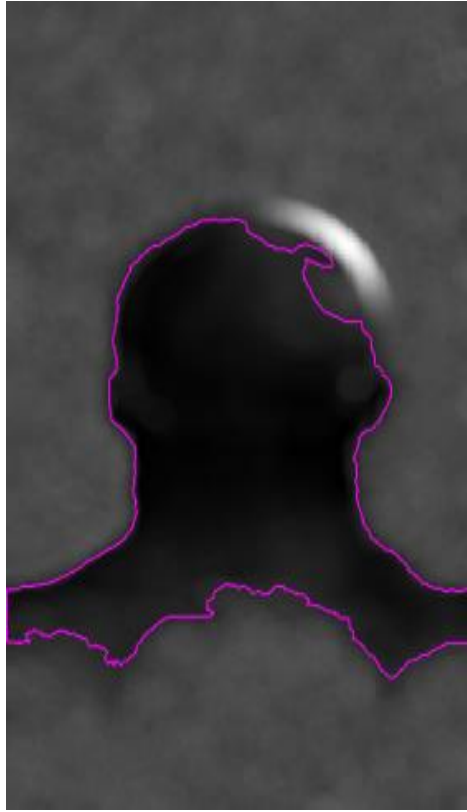
Figure 7: Segmentation based on the standard deviation filtered sensitivity image of a single coil element
