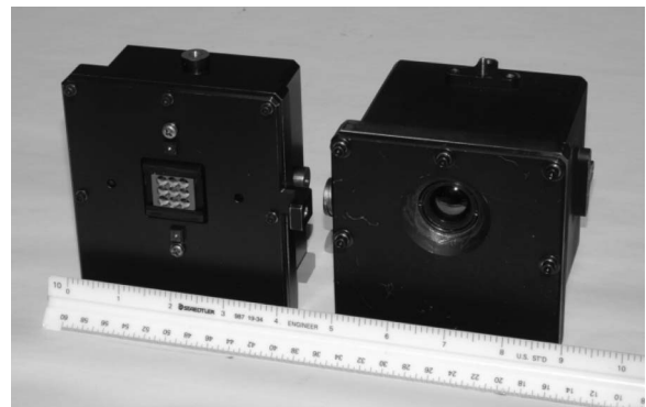
Fig. 3. Multichannel infrared camera (left) used to demonstrate compressive measurements for video. It contains a 3 \times 3 lenslet array to create nine nonredundant low-resolution images of the scene. Video from a conventional single-aperture infrared camera (right) is used to compare the quality of the video reconstructions.
