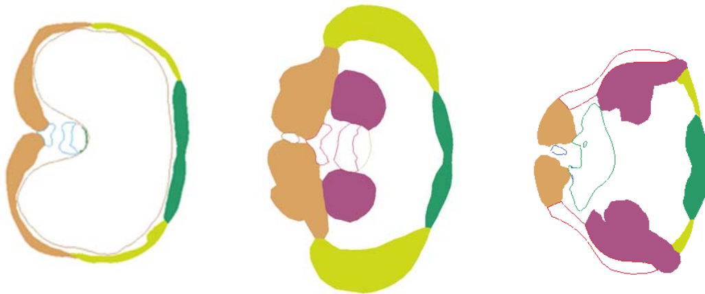
Figure 20. Model transverse cut planes at joint centers of rotation. Left- T12L1, middle- L4L5, right- L5S1. Solid elements in full color, with shell parts outlined.
