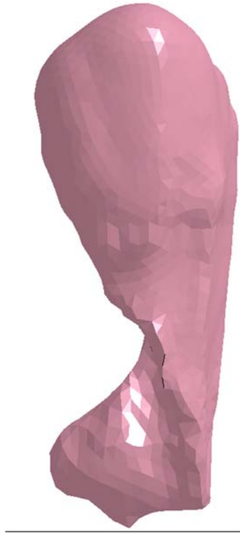
Figure 11. Abdominal volume solid mesh which is bound by and contoured to the diaphragm superiorly, pelvis and pelvic floor inferiorly, abdominal muscles anteriorly, and spinal muscles and spine posteriorly. This part is used to initialize the mean intra-abdominal pressure.
