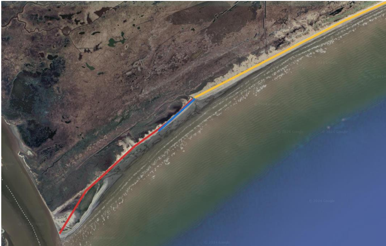
Figure 3. Yellow line indicates accessible survey area. Red line indicates area that is inaccessible. Blue line indicates UAS VLOS extended survey potential. Produced with Google Earth.
