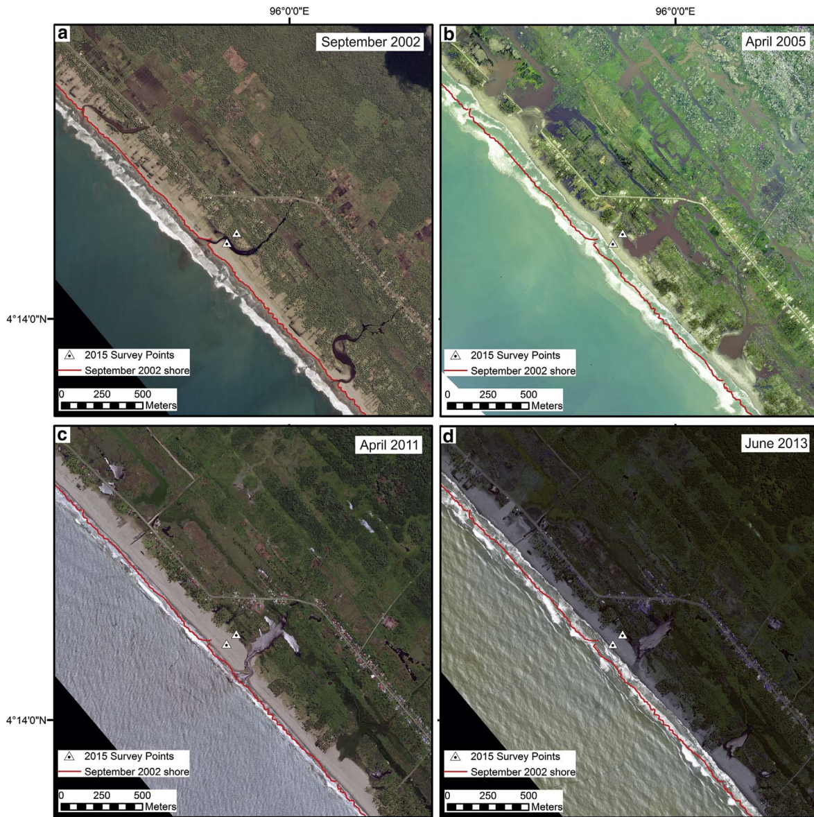
Fig. 2. Detail of Fig. 1b showing pre-tsunami conditions (i.e. 2002) and post tsunami coastal development. Red line marks 2002 shore in all images. Triangles indicate location of beach surveys (see Fig. 3) and mark top of beach ridge and most seaward swale in 2015. April 2005 and 2011 images were taken towards the end of the East Monsoon season; 2002 and 2013 images during the more energetic West Monsoon. Satellite imagery is from Quickbird (2002), World-View-2 (2011) and Pleiades (2013). 2005 aerial photographs are from the SIM Center of the Aceh and Nias Rehabilitation and Reconstruction Board (BRR).
