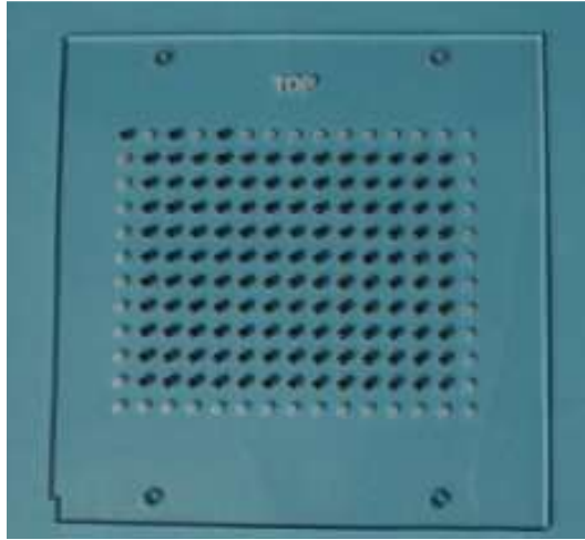
Figure 2-6: Photograph of beam stop array (BSA) developed by Dr. Priti Madhav used for scatter correction. The BSA is a 9.5x9.5x2mm acrylic plate that consists of 108 2mm diameter lead balls spaced 5mm apart in 2-dimensions on a Cartesian grid.
