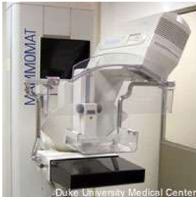
Figure 1-5: Photograph of the Duke University Medical Center prototype breast tomosynthesis system (figure obtained from [19]).
