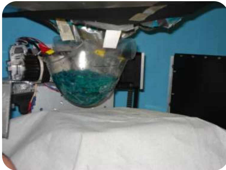
Figure 2-3: Photo of the anthropomorphic breast phantom containing acrylic yarn hanging in the MMIL system.
