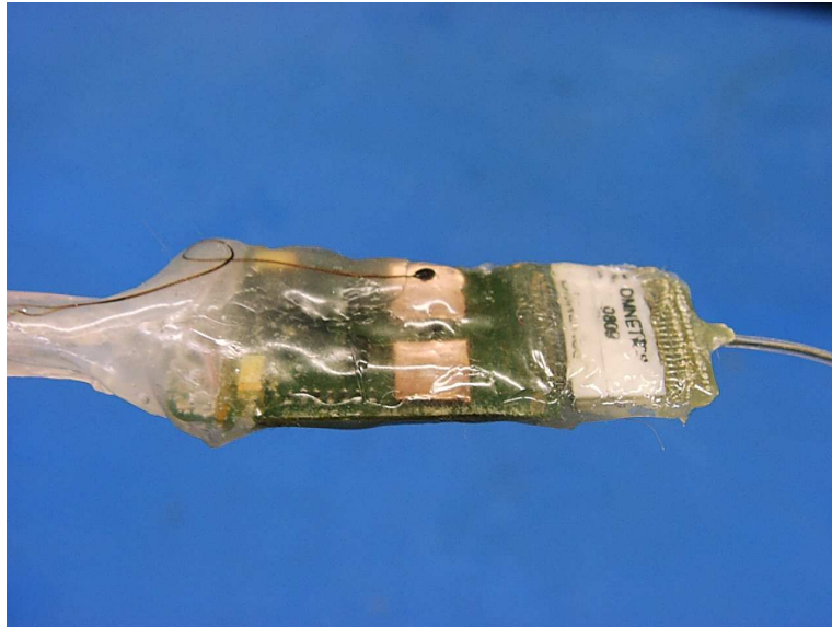
Figure 5.2: Photograph of DHSM packaged for an in vivo experiment. In the center of the board, the two analog ICs are visible, covered in copper foil for noise reduction. A thermistor is present over one of them at the outer epoxy surface. The lead wires are also visible. These wires make their way into the DHSM cable, out of the picture to the left. Also note the omnetics electrode connector and electrode cable to the right.
