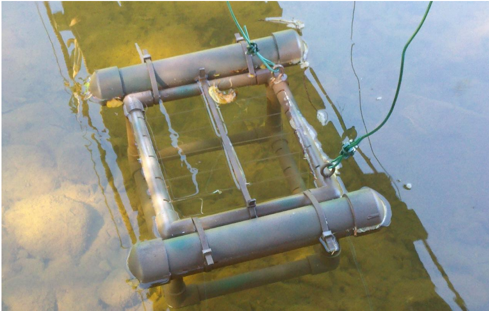
Figure 32: Biofilm rig used to collect biofilms from the Mud River, West Virginia
