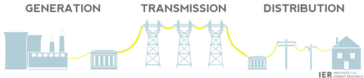
Figure 1. The three basic components of the U.S. electrical system: generation, transmission, and distribution (Institute for Energy Research, 2014).
