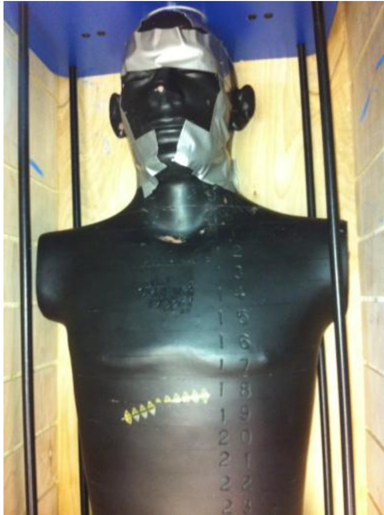
Figure 6.4: Anthropomorphic phantom used for the head and neck and lung anatomic sites.
