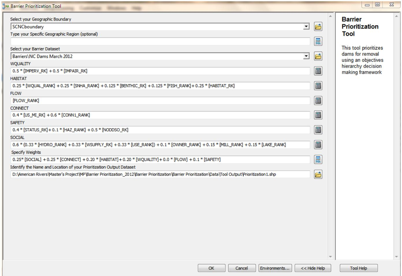
Figure 6: Model View of the Barrier Prioritization Tool in Model Builder, ArcGIS 10
