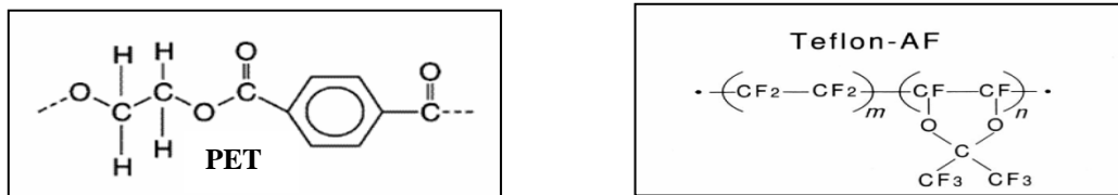
Figure 3.1. Chemical repeat structures for Mylar composed of polyethylene terephthalate (PET) and Teflon-AF. Note the structural difference in Teflon-AF compared to ePTFE structure in chapter 2.
