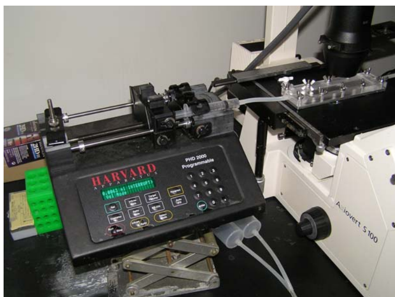
Figure 6.3. Picture of cell injection into flow chamber with a 10 ml syringe hooked up to a pump at 1 ml/min. The viewing field of the microscope is directly over the objective and is positioned at 5.2 cm from the injection point.
