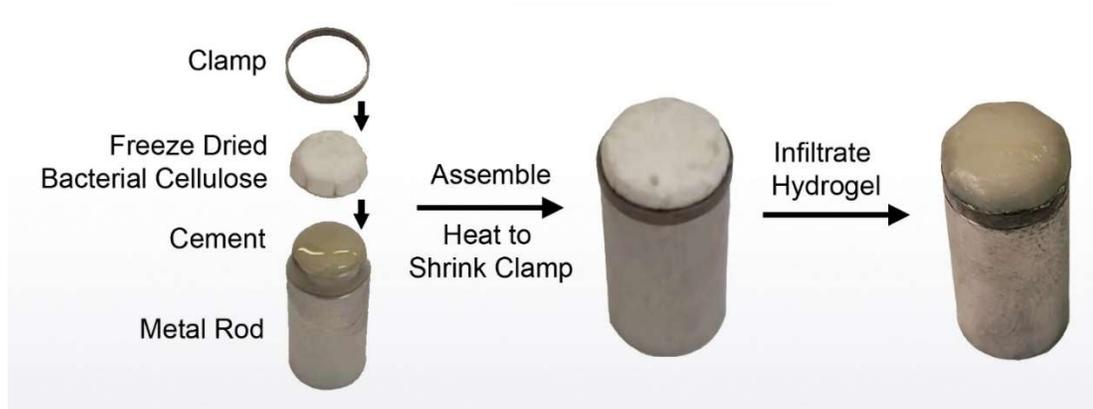
**Figure 13.** Overview of the novel method of attaching a hydrogel to a metallic plug with a shape memory alloy clamp.
