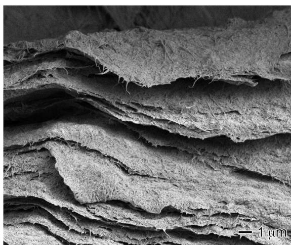
**Figure 12.** SEM image of a cross-section of a bacterial cellulose sheet.
