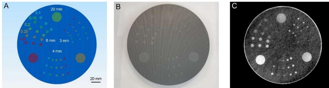
**Figure 5.** (A) Simplify 3D software image showing the dimensions of the printed areas (3 – 20 mm). The different colors in (A) represent different printing processes with extrusion multipliers of 0.1, 0.15, 0.2, 0.25, 0.3 respectively. (B) Optical image of the contrast detail phantom. (C) CT image with a window width of 280 HU.
