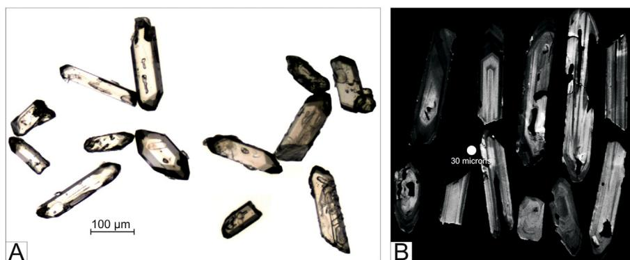
**Fig. 6.** Different views of part of the zircon population of the sample CECA-2. A) View under a transmitted-light microscope; B) Cathodoluminescence image of cut and polished grains. The size of the laser spot ( $30 \mu\text{m}$ ) is indicated.
