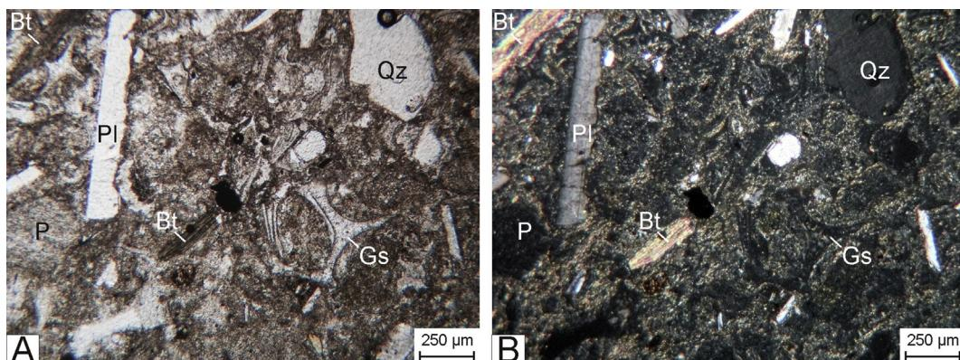
**Fig. 5.** Microphotographs of a thin section for sample RSC-27. Plagioclase (Pl), quartz (Qz) and biotite (Bt) are part of the primary crystal fragments. Glass shards (Gs) and pumice fragments (P) are partially recrystallized. Groundmass is formed by fine-grained clay mineral alteration after glass. A) Plane-parallel light; B) Crossed nicols.
