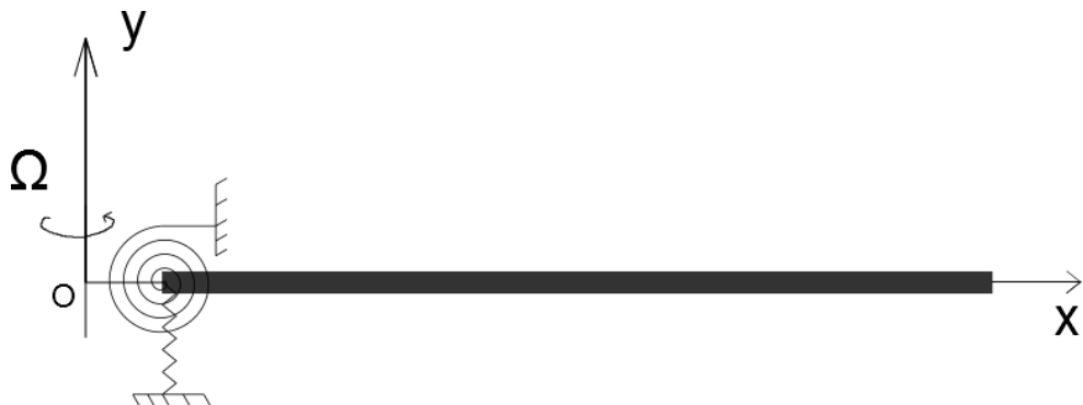
Figure 12: Coordinate system of single beam model
