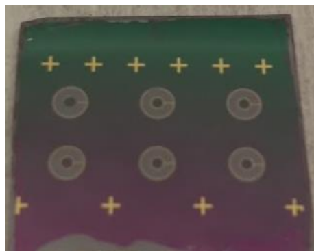
Figure 34. Thin film silicon mesas on SOI with double-ring gold top contacts.
